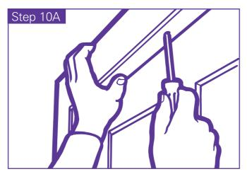
Step 10A. Screw in place the removable fillet using  $4 \times 35 \text{mm}$  screws through a white snap cap base. Finish off with supplied snap caps. Refer to Steps 10A, 10B and 10C.
