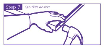
Step 7. Cut the 2 glide guide strips to suit the door width. Tack both strips to the bottom of the door using 5 panel pins with each glide guide strip.
