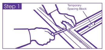
Step 1. Fit and screw the head track assembly to the cavity pocket using the 6 x 12mm countersunk screws. **Do not remove** the temporary spacing blocks until the wall sheeting has been completed. Failure to adhere will void warranty.
