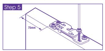
Step 5. Attach the 2 x door brackets to the top of the door using the 8 x 30mm hex head screws, 75mm in from each side and central to the thickness of the door. Ensure both door support brackets are facing in the same direction.
