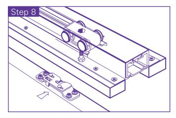
Step 8. With the door in the cavity opening, lift the door to locate each door support bracket onto the carriage assembly bolt.
