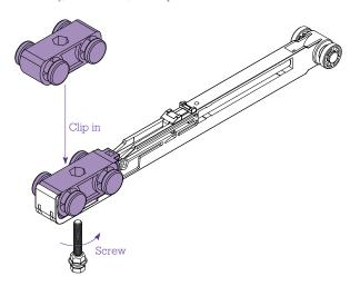
Take the bolt removed in step 2, screw the bolt through the Soft Closer and the trolley so that the door can be rehund.
